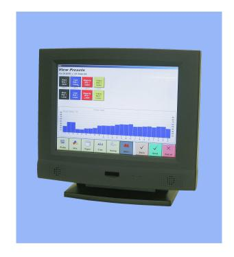
The digital image files produced by Computer-To-Plate (CTP) systems are electronically scanned to give image coverage data. Tobias EPLEX-Lite™ uses the coverage information to preset the ink fountain keys for rapid makeready and waste reduction.
